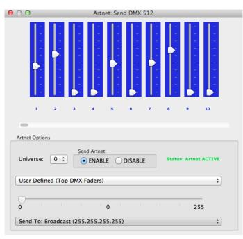
When first opened, the Art-Net is set to Disabled, please set it to Enabled, and then you can use either the DMX faders to test one or more DMX channels, or use the testpatterns from the options available.
