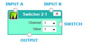
Switcher 2-1: Controllable Switch operator, acts as a normal Input A to Output Action, but when the trigger value is greater than the set Switch it does Input B to Output Action
